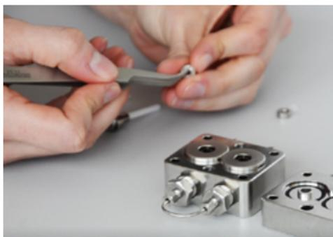
**Fig. 13:** Separating backing ring and adjusting ring
