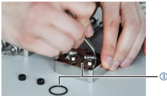
**Fig. 18:** Removing o-rings
