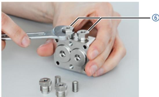
**Fig.22:** Removing lower bushings
