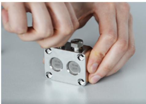
**Fig.27:** Inserting bushings
