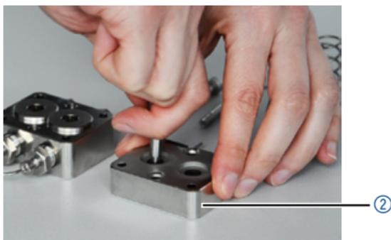
**Fig. 17:** Removing seals (low-pressure side)
